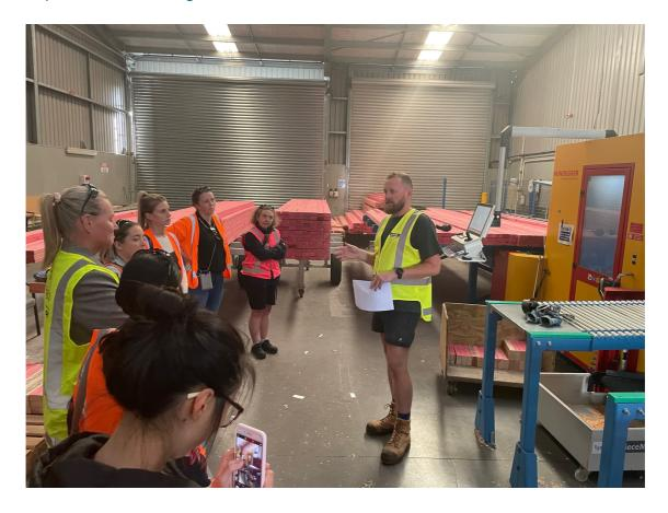
Carters Cambridge factory manager Aaron Quinn explains the operation of the Hundegger optimising saw to the NAWIC group – the first step in converting timber stock into finished frames and trusses.
